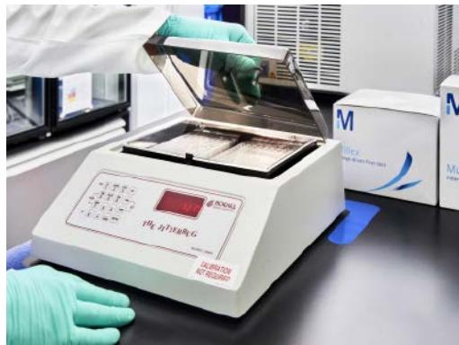
The microplate shaker is temperature controlled and ideal for immunoassays like SMC™. Includes an inner lid to eliminate light and reduce the risk of contamination.
