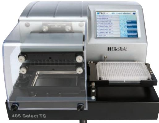
In partnership with BioTek®, we offer the latest advancements in 96-well plate washing: a fully automated system designed to quickly wash an entire plate through biomagnetic separation, washing and vacuum filtration. The system comes specifically optimized for use with SMC™ assays with the inclusion of a specially designed magnetic plate and customized pre-programmed plate washing protocols. The 405™ TS model offers an easy-to-use and glove touchable screen.
